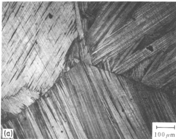
Figure 6 Optical microstructures of Cu-14.2Zn-8.5Al shape-memory alloy: aged for (a) 1 h at 300° C, (b) 15 min at 400° C, (c) 30 min at 500° C.
